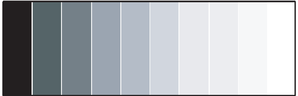
Figure 4-3. Typical Gray Bar Pattern for Adjusting Contrast
